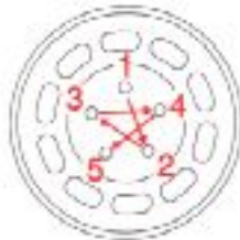
Correct tightening order for wheel bolts
