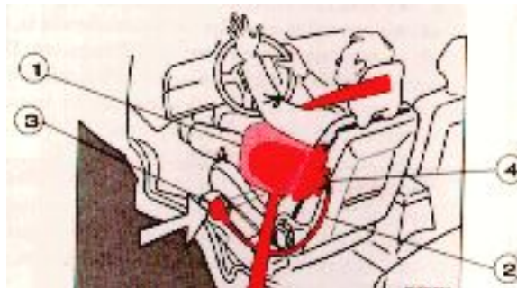
1 - Airbag, 2 - lead, 3 - sensor unit, 4 - gas generator
